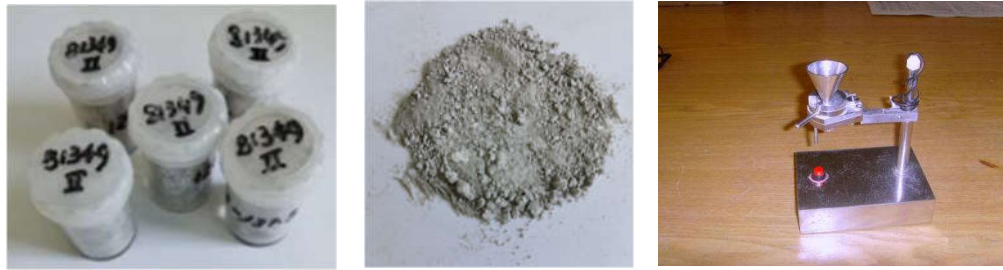
Figure 2. Calcareous biological ooze sample and sample splitter used in this study.
