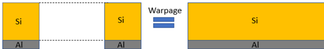
Fig.2 Annular plate and plate have the same curvature and deflection
