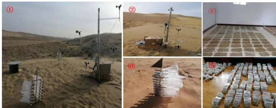
①Observation field instrument layout;② weather station(HOBO);③Sand collector;④~⑤Soil sample
