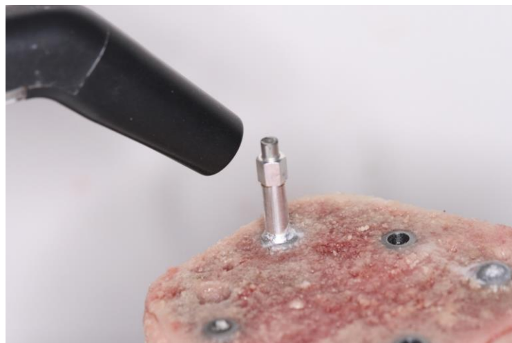
Figure 3. ISQ measurement of implant placed in the porcine tibia.
