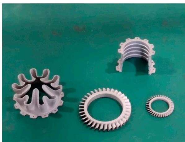
Figure 3. The small engine parts produced by Anhui Tuobao Additive Manufacturing Technology Co., Ltd. using SLM.
