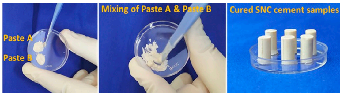
Figure 3. Preparation of shell nacre cement samples; Equal amount of paste A and paste B were mixed together and filled in the mold to get the cured samples of specific dimensions. Here the cured compressive strength samples were shown.
