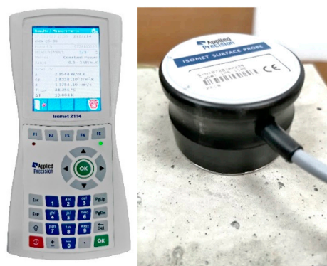
Figure 2. Measure the thermal conductivity values of the samples with the ISOMET 2114.
