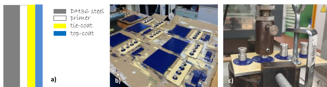
Figure 1. scheme of layers deposited on the DH36 steel (a); image of the painted steel samples for the mechanical adhesion tests (b); image of the experimental set-up for the pull-off test (c).
