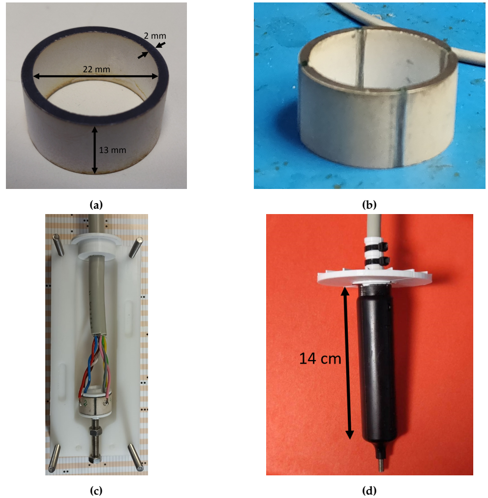
Figure 3. Prototype manufacturing: (a) piezoceramic hollow cylinder made of PZT-4; (b) piezoceramic cylinder, with eight aligned rips; (c) prototype of the spiral source in the potting frame, before the polyurethane potting; and (d) prototype of the spiral source after the polyurethane potting, with a bearing angle reference frame on the top.
