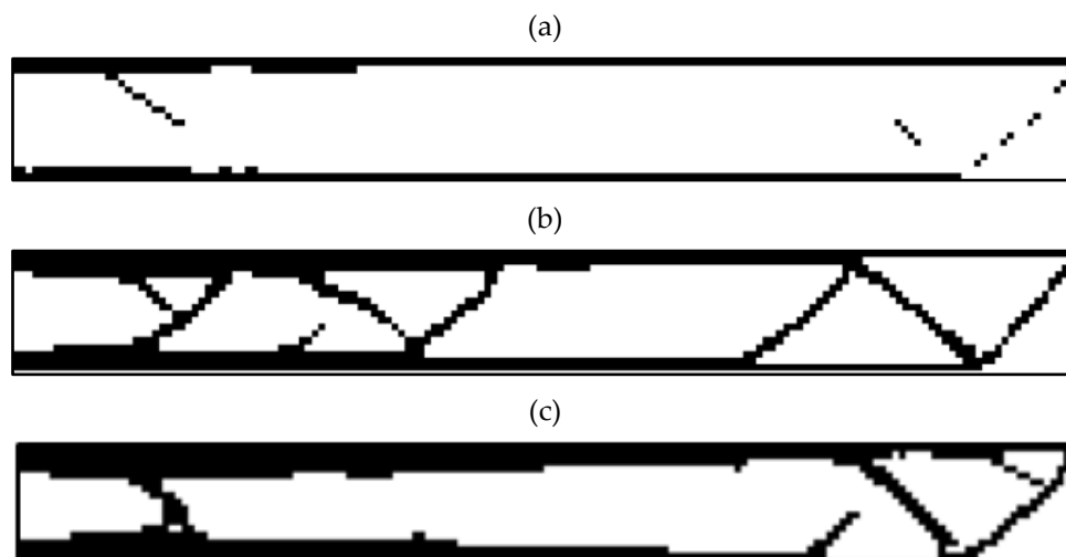
Figure 11. The results for the optimization of the rectangular plane in terms of (a) 20%, (b) 40%, and (c) 60% for the weight constraint
