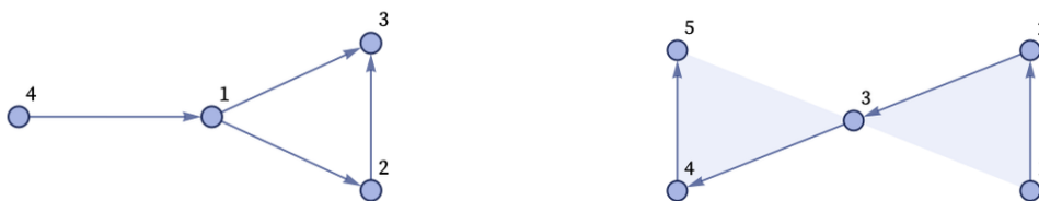
Figure 40. Two elementary examples of directed spatial hypergraphs, corresponding to the collections of ordered relations \{\{1, 2\}, \{1, 3\}, \{2, 3\}, \{4, 1\}\} and \{\{1, 2, 3\}, \{3, 4, 5\}\} , respectively.
