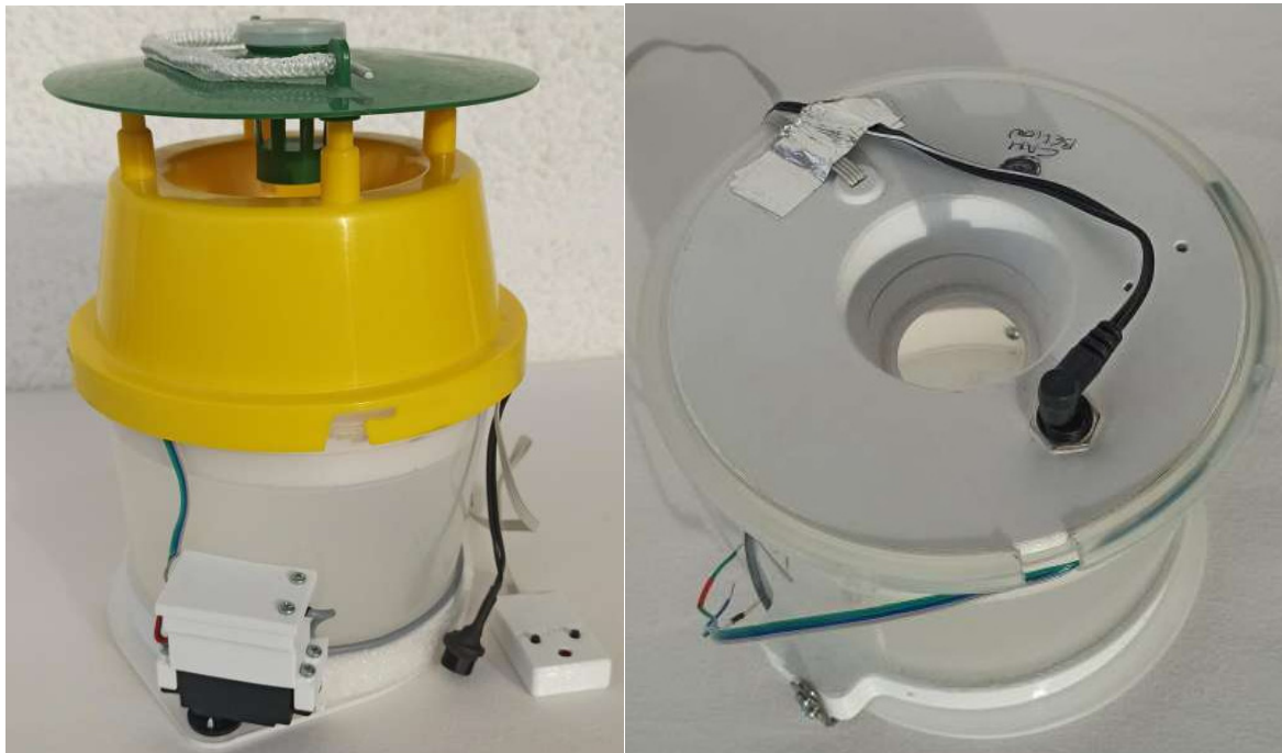
Figure 1. (Left) The camera-based funnel trap, (Right) The torus allows the electronics and camera to sit on top of the funnel trap and does not need a customized bucket.
