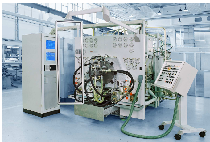
Figure 4. Hydraulic testbench with mounted pump and attached sensors (source: Bosch Rexroth AG)
