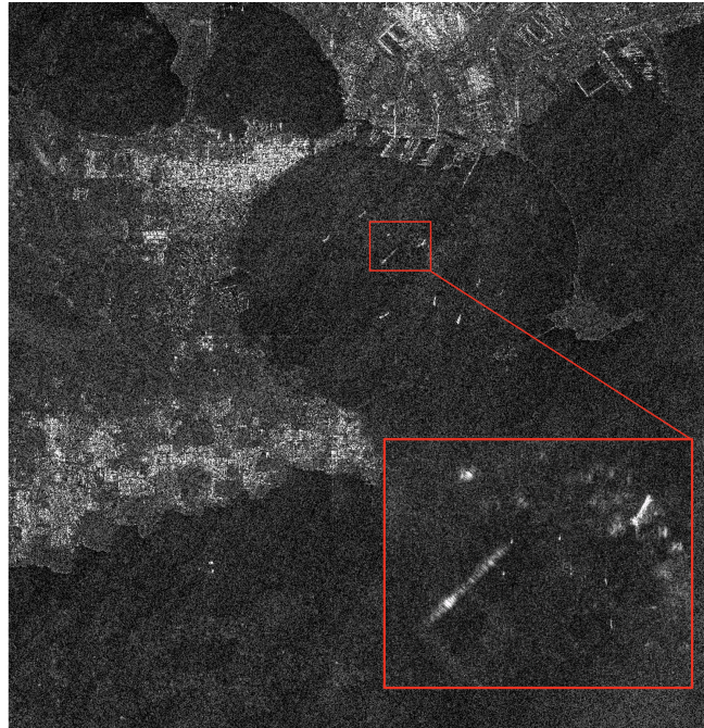
Figure 9. Test case of the CFAR+SLA algorithm over the port of Taranto. Highlighted detail: a probable radio signal transmitted from a ship and captured by X-band. [Product ID: CSKS1_SCS_BHI_05_HH_RD_SF_20200323164522_2020032316_4529 processed by University of Naples Federico II under the COAST license of the Italian Space Agency (ASI); Original COSMO-SkyMed Product - ©ASI - (2020).
