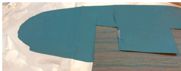
Figure 3. Anode material spread on phosphor sheet.
