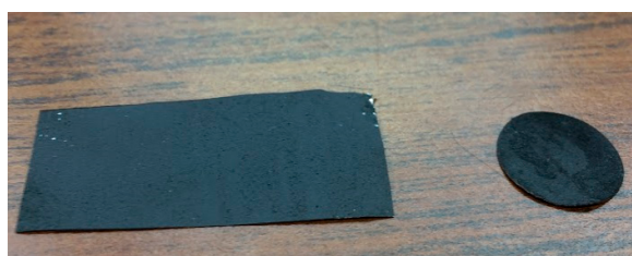
Figure 2. piece of cathode before rolling, and the cathode circle is ready to use.
