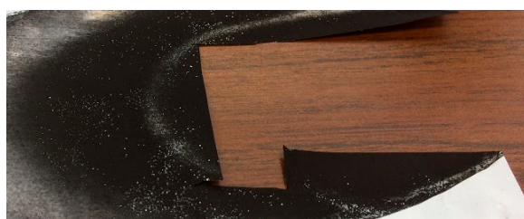
Figure 1. Cathode material spread on an aluminum sheet.
