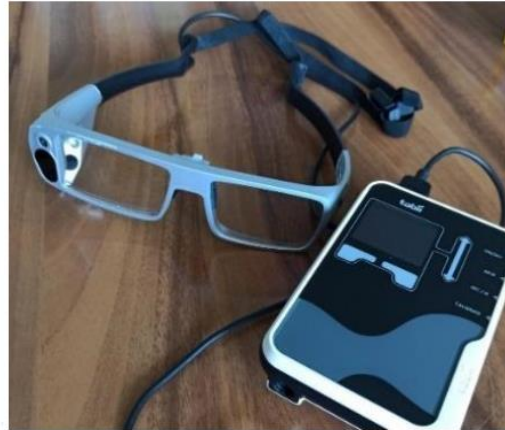
Figure 3 – The Tobii Glasses Eye Tracker® (v. 1.0) used during testing for tracking and processing of eye movements.
