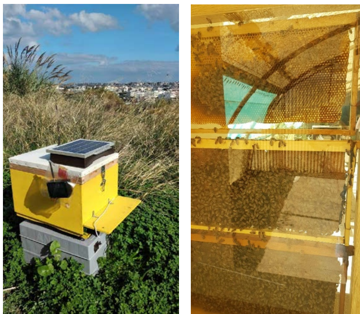
Figure 1. Beehives monitored in the course of this work with a number of sensors. (Left) The e-beehive in the field, (right) An observation beehive allows us to spot the queen and observe the patterns of activity inside it.
