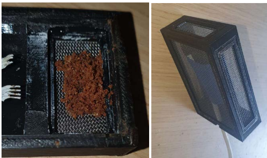
Figure 9. (Left) The bees covering the gas sensor with propolis on the left. We left only partial coverage as it was totally covered. (Right) New, gas-penetrated box houses the gas sensor and placed in the beehive in a way that not all sides can be covered by propolis.
