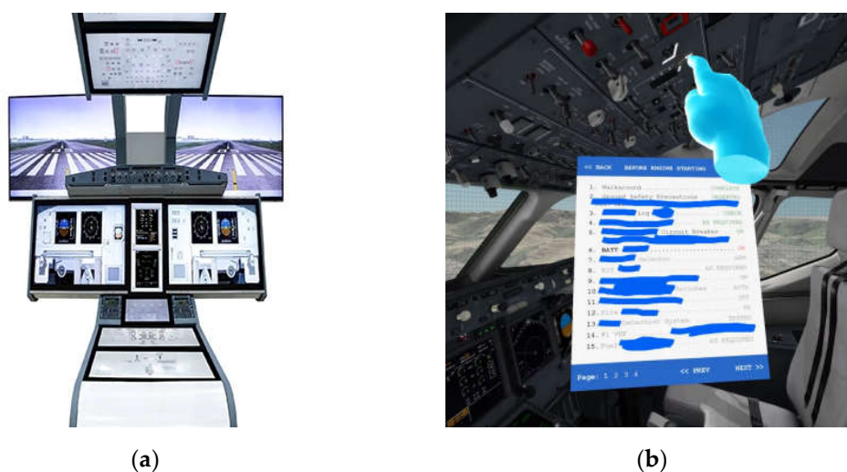
Figure 1. Two approaches to flight simulators. (a) It is possible to simulate a portion of the control surfaces with multi-touch screens and physical controls [22]; (b) It is possible to simulate the entire cockpit of an aircraft with a VR headset and interact with all control surfaces with haptic VR gloves [23].
