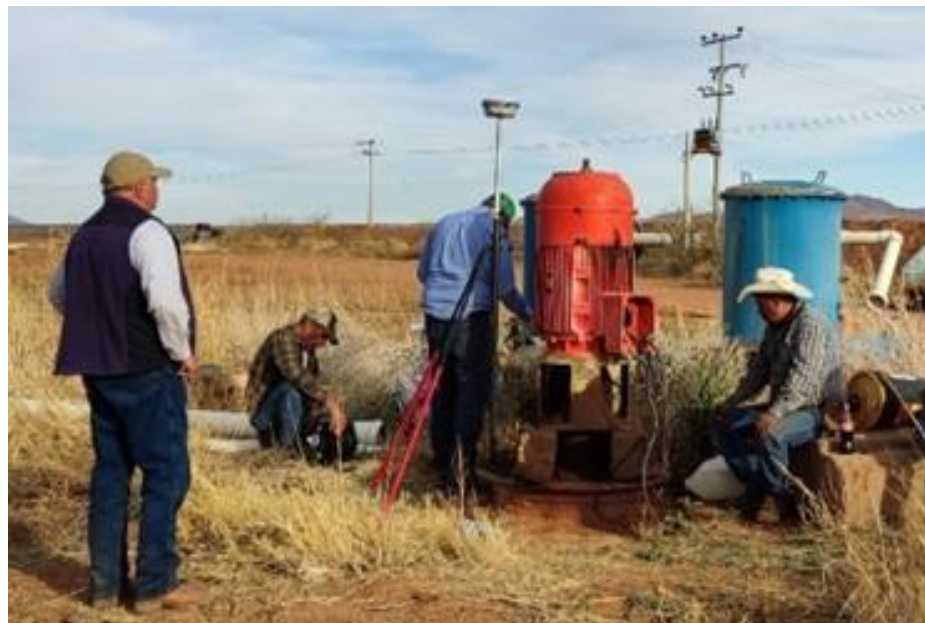
Figure 3. GPS RTK survey and evaluation of groundwater level
