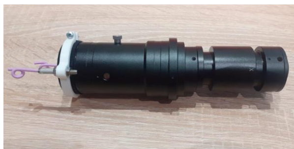
Figure 32. Lens set already with a textile yarn holder.
