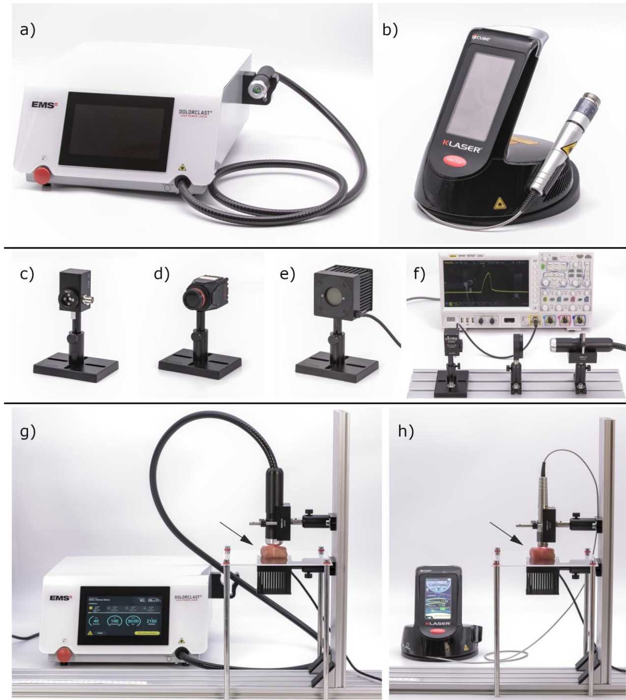
Figure 1. Laser therapy devices, sensors and experimental setups used in the present study: (a) EMS laser (Dolorclast High Power Laser; Electro Medical Systems, Nyon, Switzerland); (b) K-laser (Cube 4; Eltech K-Laser; Treviso, Italy); (c) Fast Photodiode (FPD-VIS-300; Ophir Spiricon Europe, Darmstadt, Germany) for temporal beam characterizations; (d) experimental setup for laser pulse characterization measurements with the handpiece of the EMS laser (right), the FPD (left) and an optical diffuser in the beam line (center); the FPD is connected to an oscilloscope (MSO7024; Rigol Technologies, Suzhou, China); (e) beam profiling camera (LT665; Ophir Spiricon Europe) that can measure spatial power density maps; (f) thermal power sensor (50(150)A-BB-26-PPS; Ophir Spiricon Europe); (g) experimental setup for penetration depth measurements with the EMS laser; (h) experimental setup for penetration depth measurements with the K-laser. The arrows in (g, h) point to a tissue specimen (15 mm thick chicken muscle tissue) on the specimen holder.
