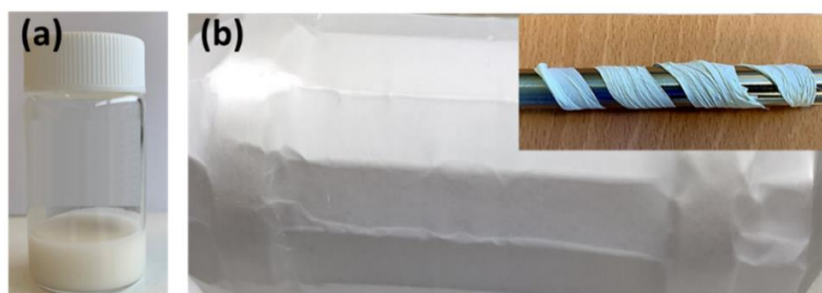
Figure 3. Perovskite polymeric solution (a) and MDABCO-NH 4 I 3 @ PVC electrospun nanofiber mat (b) the inset shows a fiber mat folded around a cylindrical stick, demonstrating the flexibility of the fibers.
