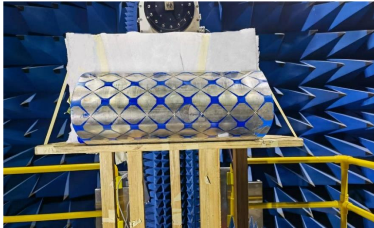
Figure 9. Test setup in the microwave anechoic chamber, z-axis point to the top of the antenna.
