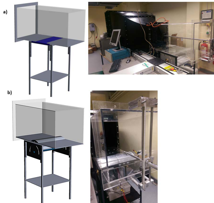
Figure 6: a- benchmark wind tunnel configurations (solid works and real setup) b-convex hump attached to the wind tunnel test section (solid works and real setup).
