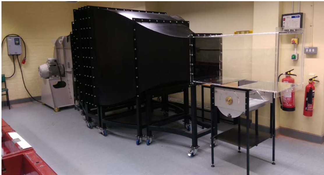
Figure 5: The final constructed layout of the built open-jet wind tunnel.
