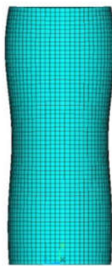
Figure 6. Magnified view of local imperfections.
