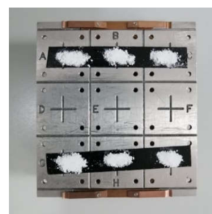
Figure 2. Samples placed on the plate for respective analysis by XPS.
