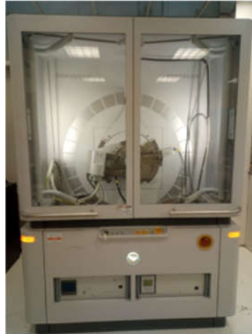
Figure 3. X-ray diffractometer model Panalytical Empyrean
