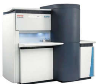
Figure 1. XPS Thermo Scientific Inc. Model K-Alpha.
