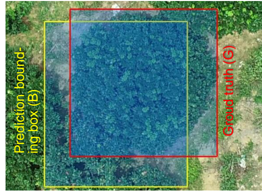
Figure 8. Intersection over the union of ground truth and prediction bounding box.
