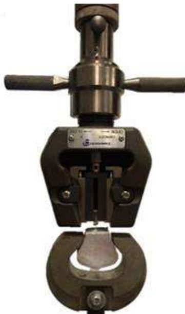
Fig. 2 The pullout test setup
