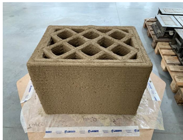
Figure 5. 3D printed specimen in the fresh state.
