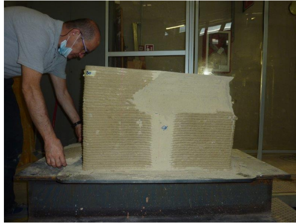
Figure 12. Front view of the specimen after the load test, with the upper face permanently inclined from left to right.
