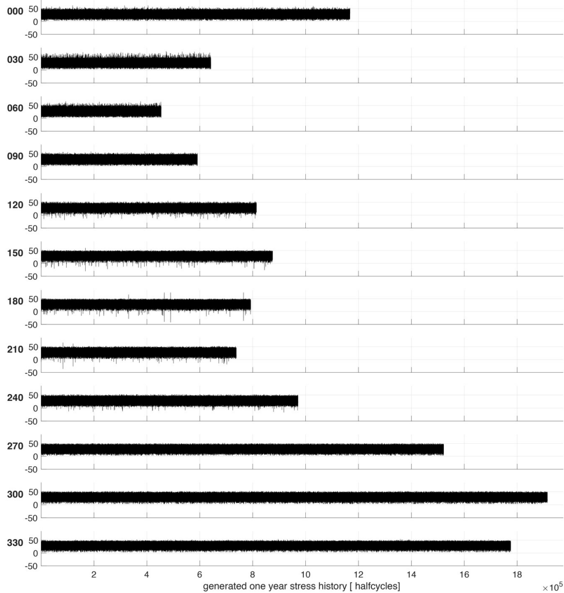
Figure 8. Random load cycles of one-year duration obtained from the Markov chain method for all 12 sectors with an applied omission level of 10%
