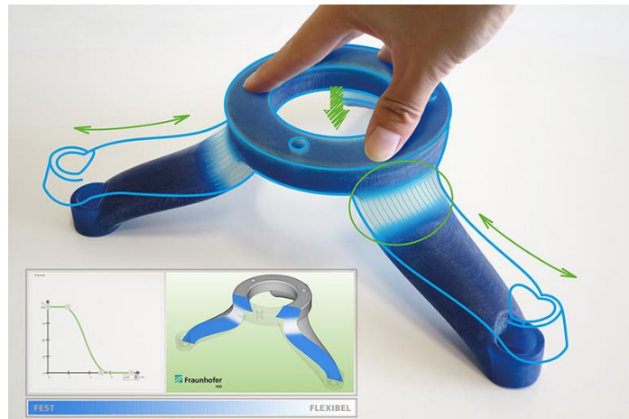
Figure 17. Interactively designed multi-material sample part using GraMMaCAD software developed by the Fraunhofer Institute [124].
