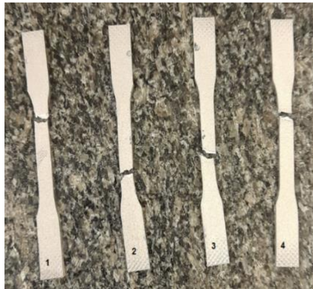
Figure 7: Fractured tensile test specimen
