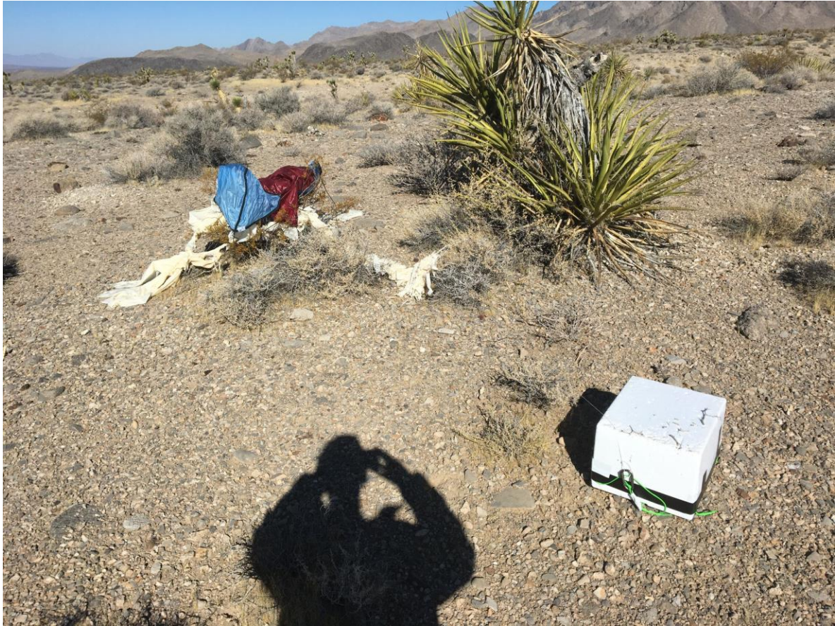
Figure 2. Landing site, with payload box flipped upside down on the lower right and the parachute (blue and red) tangled with balloon shreds in the upper left.
