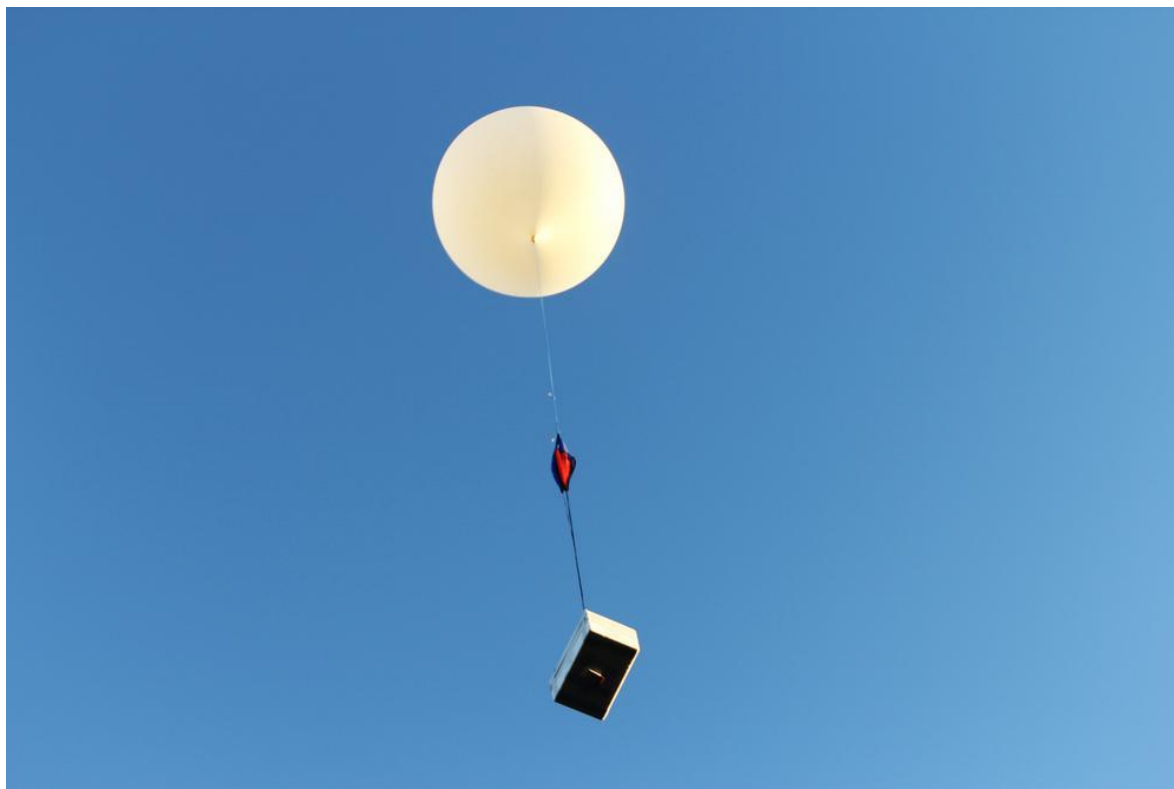
Figure 1. A meteorological balloon carrying infrasound sensors in a PolarTech insulated shipping container in 2015. The parachute is visible between the box and the balloon. The Skyfall setup is very similar to the one described here.
