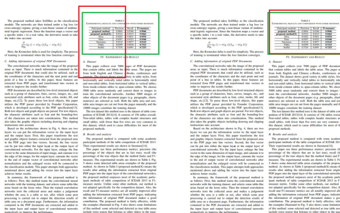
Figure 10. An instance of a precise and imprecise table detection. Green color represents the ground-truth tabular area whereas red color denotes the predicted tabular boundary.
