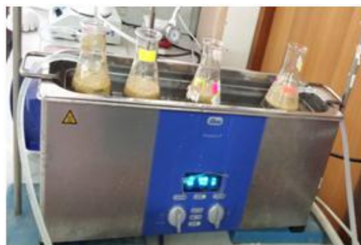
Figure 1. The experimental setup used for US pretreatment.
