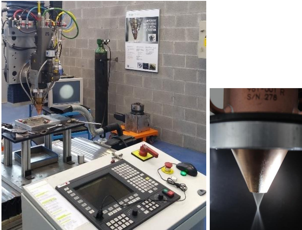
Figure 2. Cartesian kinematics LMD station in LORTEK. Detail of the station (left) and detail of the Coax40 nozzle with the powder flow (right).
