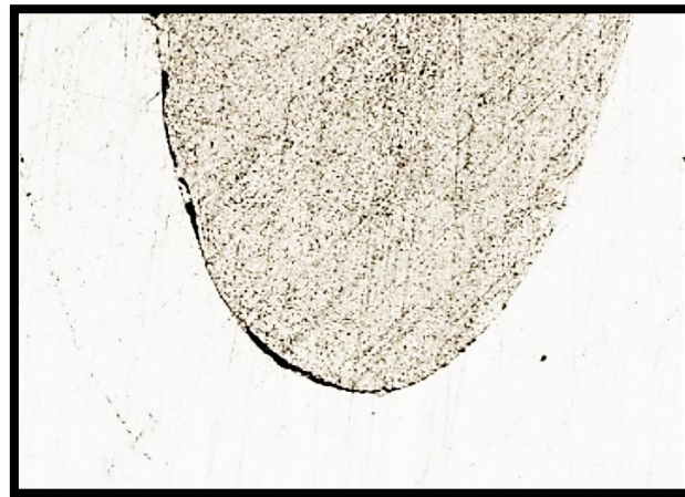
Figure 9. Imperfections (black areas) at the end of the wavy borderline of the joint
