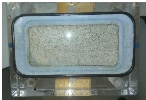
Fig. 12. Photo of membrane support after using 7% solution MNP as a DS.
