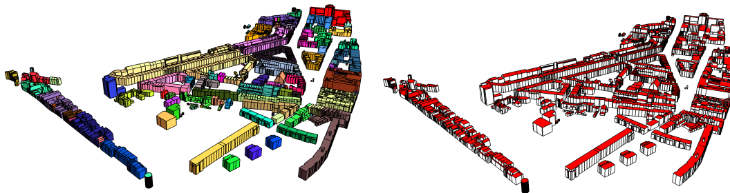
(b) All facets (2-cells) that are incident to the same volume (3-cell) have the same colour. This figure highlights the topological characteristics of the dataset and shows that multiple semantically individual buildings have been merged, topologically, under the same volume.
