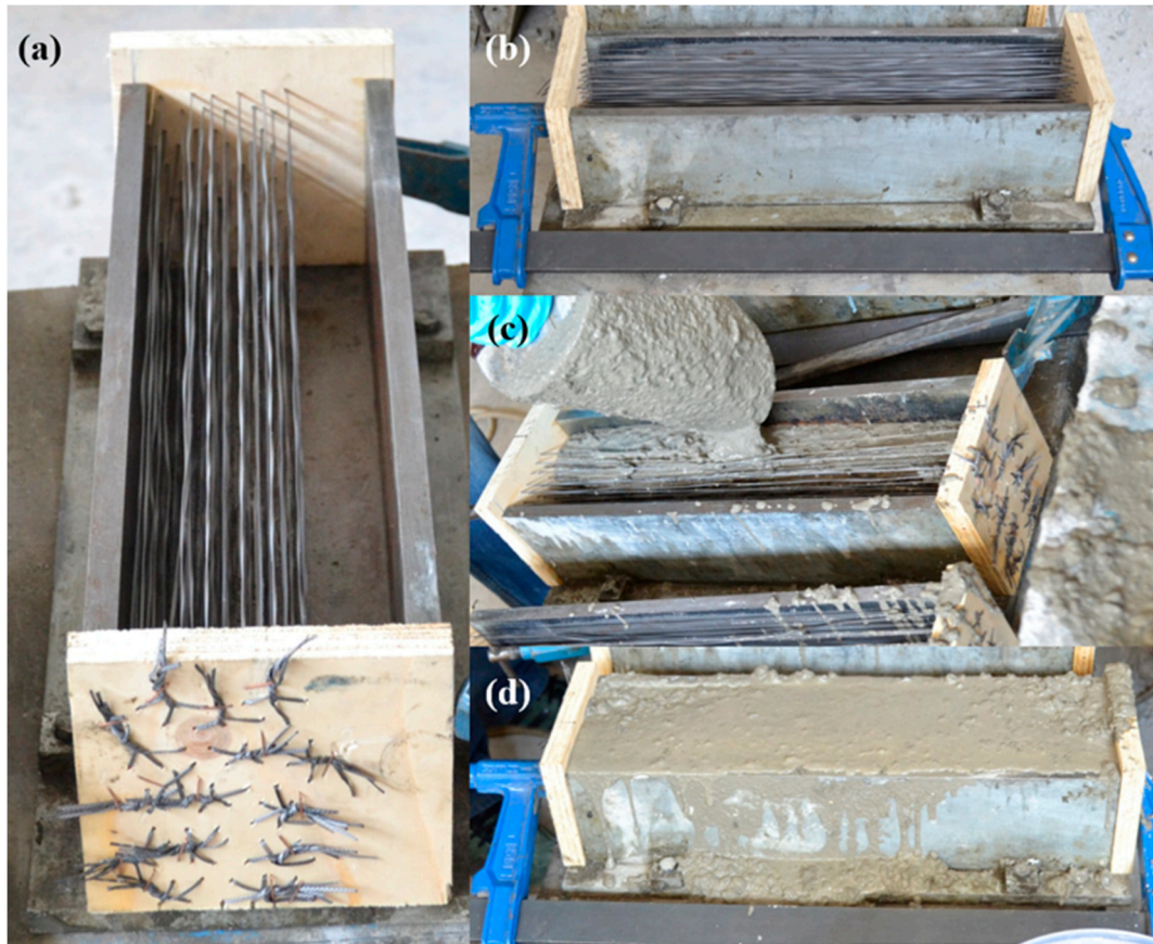
Figure 3. (a) Positioning of the long fibres in the moulds; (b) fixing the mould sides to avoid any damage in the fibres while concrete in fresh state; (c) Pouring of self-compacting concrete; (d) final appearance of the specimens.
