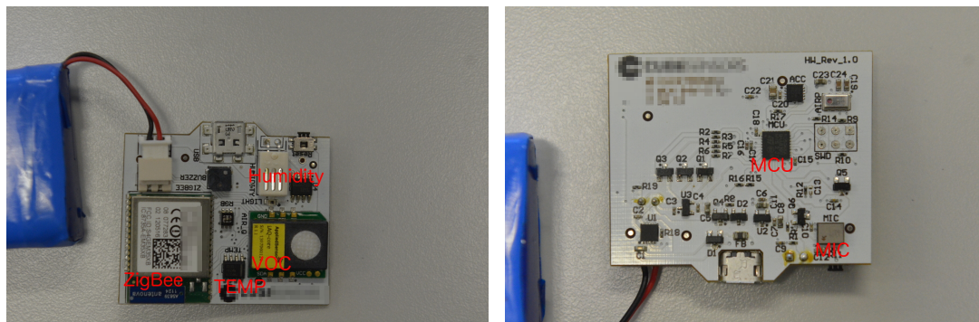
(a) The top side of the node's PCB. It contains the humidity sensor, the VOC sensor, the temperature sensor and the ZigBee transceiver.
