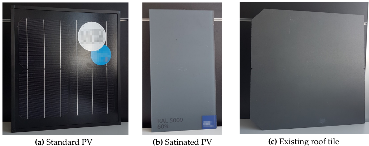
Figure 7. Photographs of material samples used in the case study: standard PV (a), satinated PV (b), and existing roof tile (c).
