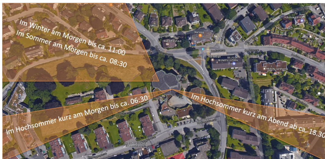
Figure 3. Reflection zones and timespans from roof of St. Michael's church predicted by PV system installer for initially proposed PV roof retrofit. Image courtesy of BE Netz AG.
