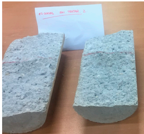
Figure 6. Penetration of water under pressure, M4.
