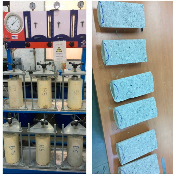
Figure 2. Depth of penetration of water under pressure (a) test and (b) specimens.
