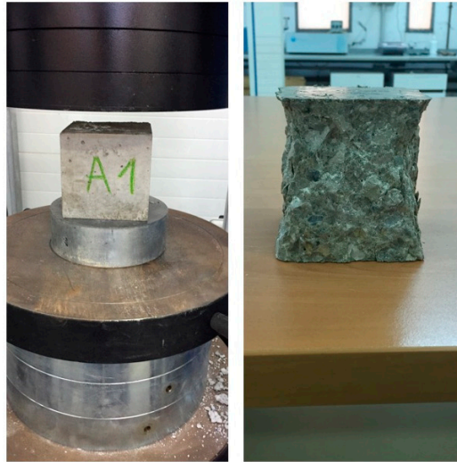
Figure 1. Compressive strength (a) test and (b) specimens.
