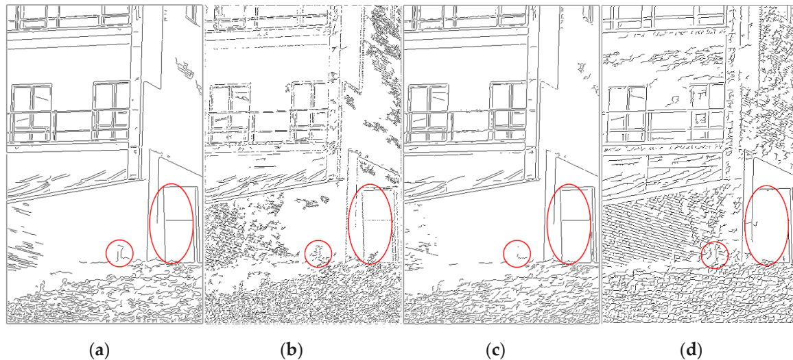
Figure 15. The binary edge maps generated for the Scene 7 by (a) GEDHSI, (b) Di Zenzo's method, (c) the RCMG method and (d) Drewniok's method ( \sigma = 1.0 ).
