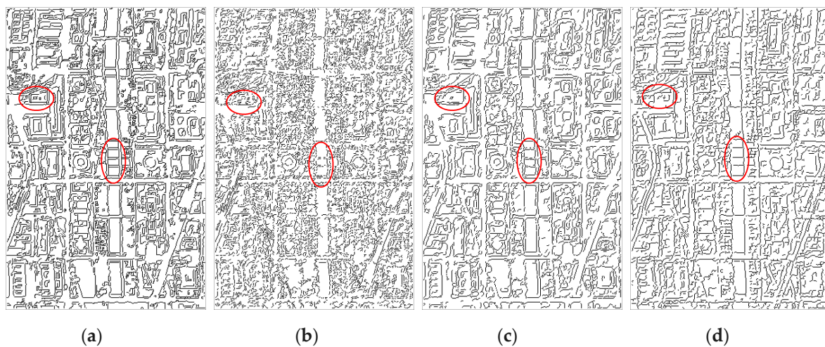
Figure 12. The binary edge maps of the Washington DC Mall by (a) GEDHSI, (b) Di Zenzo's method, (c) the RCMG method, (d) Drewniok's method ( \sigma=1.0 ).
